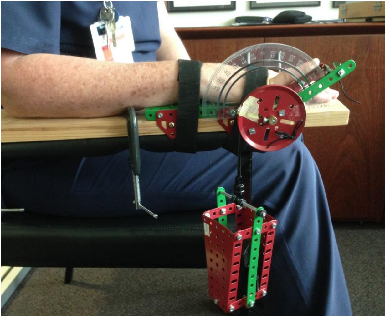
Figure 5: The Hunter Hyperextensometer in use. The device has been constructed from Meccanno. The participant's wrist and metacarpophalangeal joints are secured in apposition to the platform. A fixed torque is applied to passively extend the 5 th metacarpophalangeal joint by placing 600 grams of weights in the Meccanno cradle suspended from the pulley wheel (radius 35 mm) to deliver a torque of 2.59 N cm. The angular displacement in response to this standard torque is measured in degrees of extension after 60 seconds.
