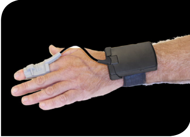
Figure 2: AliveLock RiskWatch wrist-worn device and finger sensor
